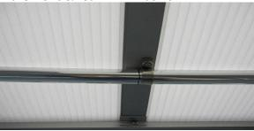
Apply a small bead of clear caulk to the inside corner of the E-8. Nest the side channels (E-8 edge) of polycarbonate sheets and locate over the center of the Bimini cross bows as shown exploded view.
